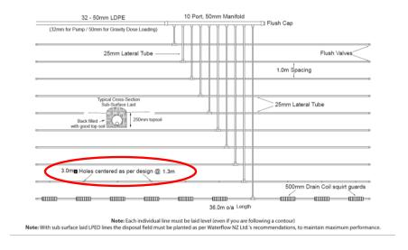
2. Clip on Squirt Guards over each hole drilled in the dripline.
