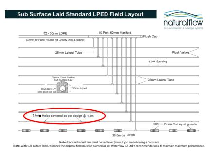
2. Clip on Squirt Guards over each hole drilled in the dripline.
