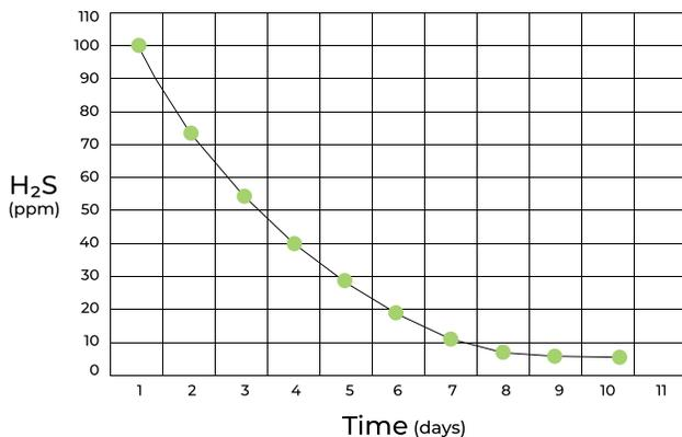
H<sub>2</sub>S measurements in wet wells and downstream manholes reduced 80–97%.
